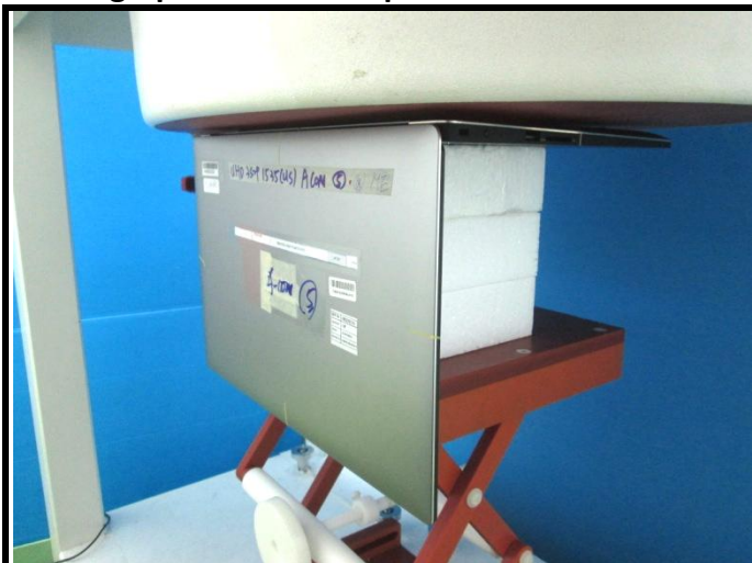
Bottom of EUT with 0 cm Gap (EUT 1 with Antenna 1 (ACON))
