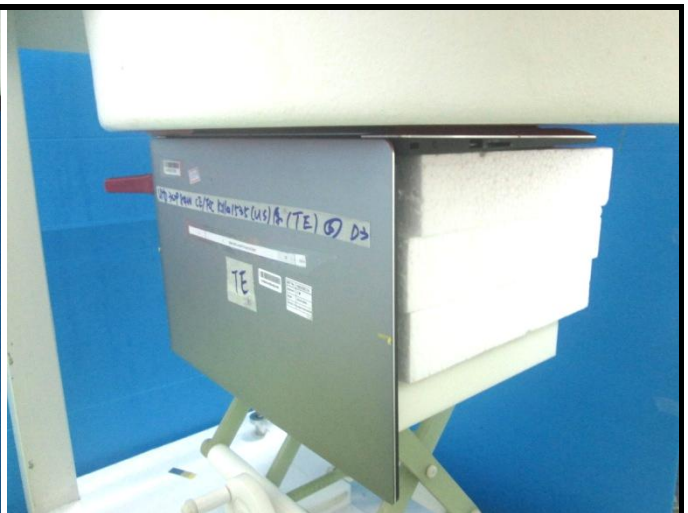
Bottom of EUT with 0 cm Gap (EUT 2 with Antenna 2 (TE))
