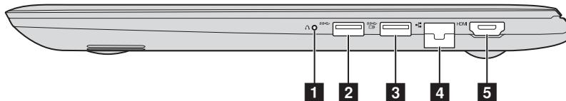
**1 Novo button** When the computer is off, press this button to start the Lenovo OneKey Recovery system or the BIOS setup utility, or to enter the boot menu.
