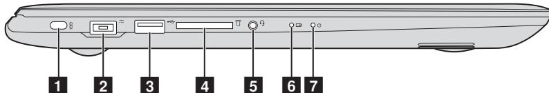
**1 Kensington slot** Attach a security lock (not supplied) here to help protect your computer from theft and unauthorized use.
