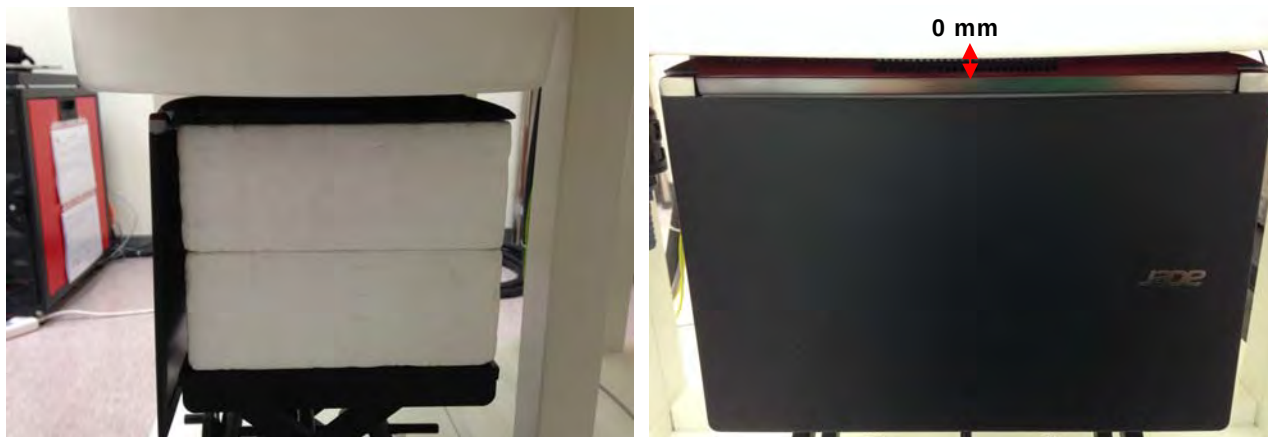
Fig.3 EUT Lap-held mode to flat phantom
