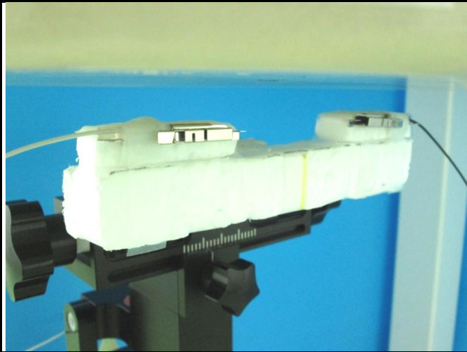
Front Face of EUT with 1.5 cm Gap
