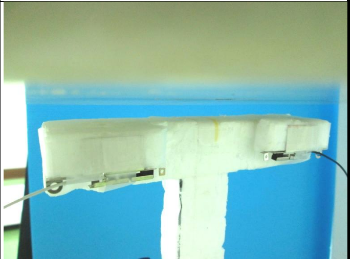
Bottom Side of EUT with 1.5 cm Gap
