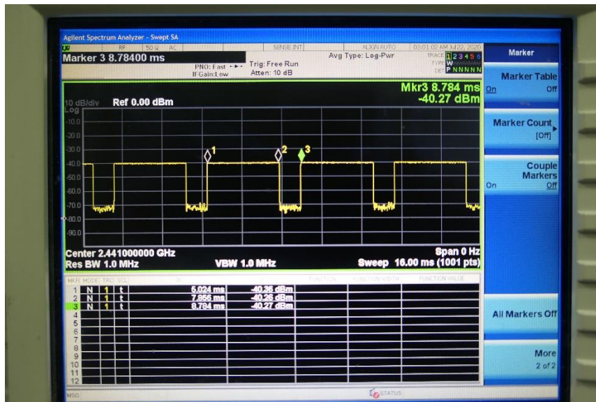
Time-domain plot for Bluetooth transmission signal
