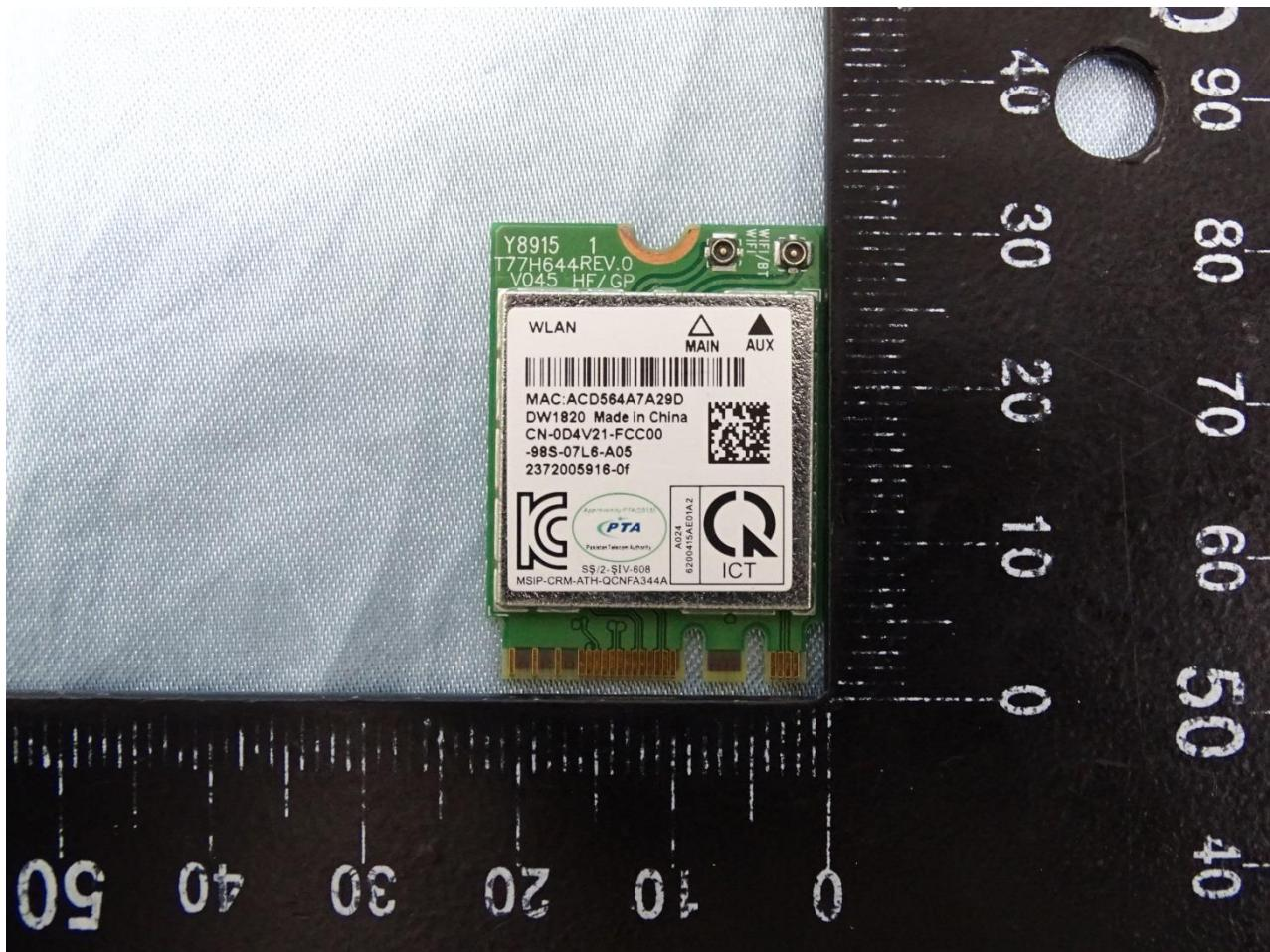
**EUT: 802.11 a/b/g/n/ac + BT 4.1 M.2 2230 Type Card**
