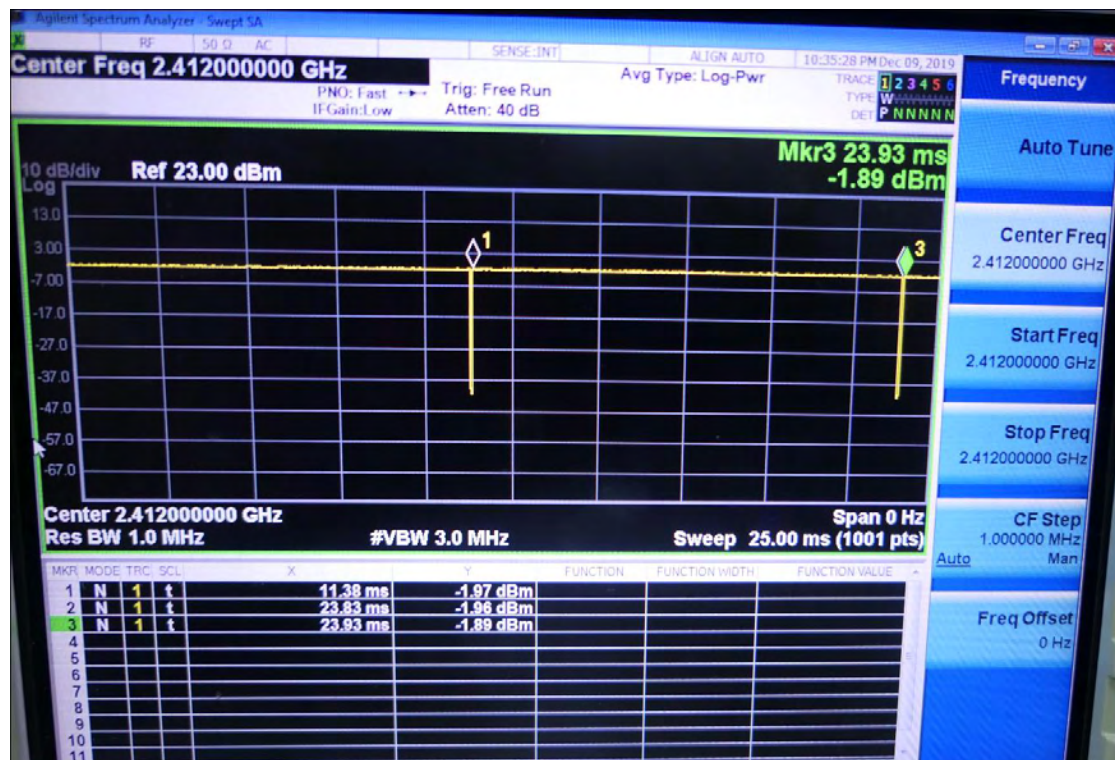
Time-domain plot for 802.11b transmission signal
