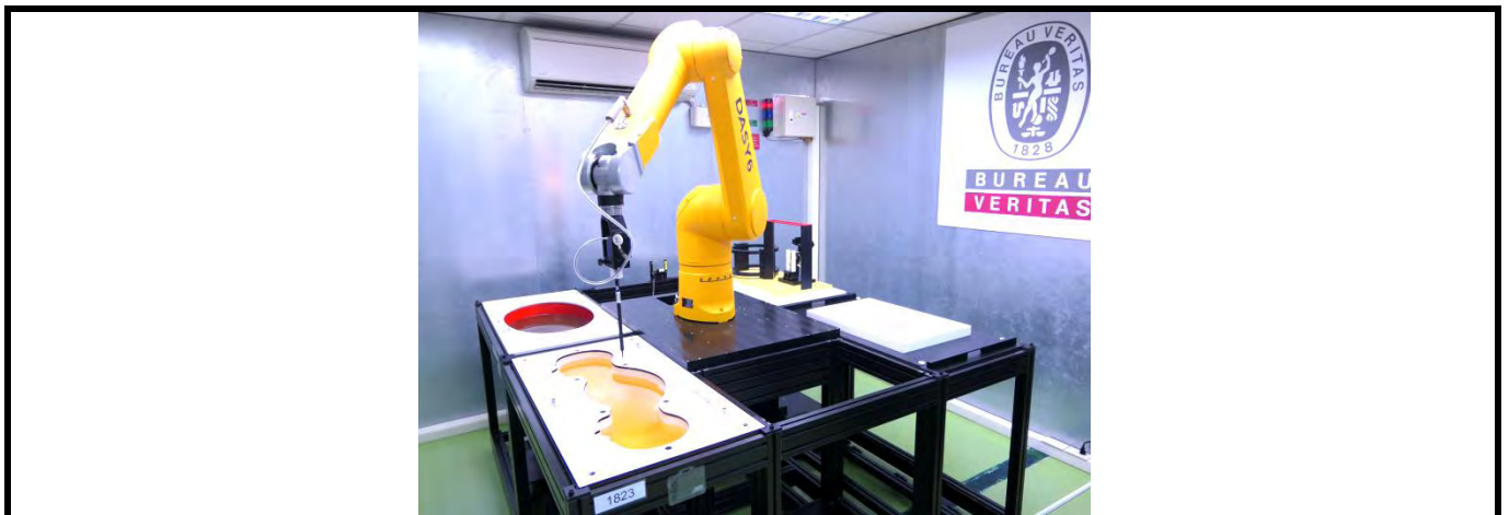
Fig-3.2 SPEAG DASY6 System
