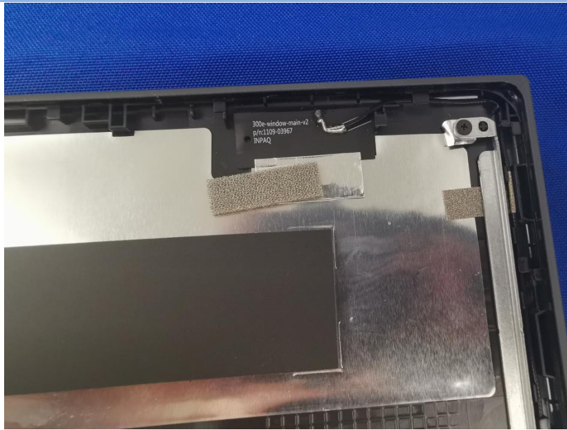
ANTENNA PHOTO (MAIN ANTENNA)
