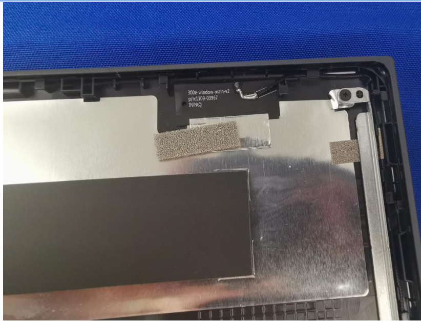
ANTENNA PHOTO (MAIN ANTENNA)
