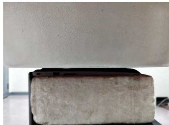
Fig.3 EUT Bottom side to flat phantom
