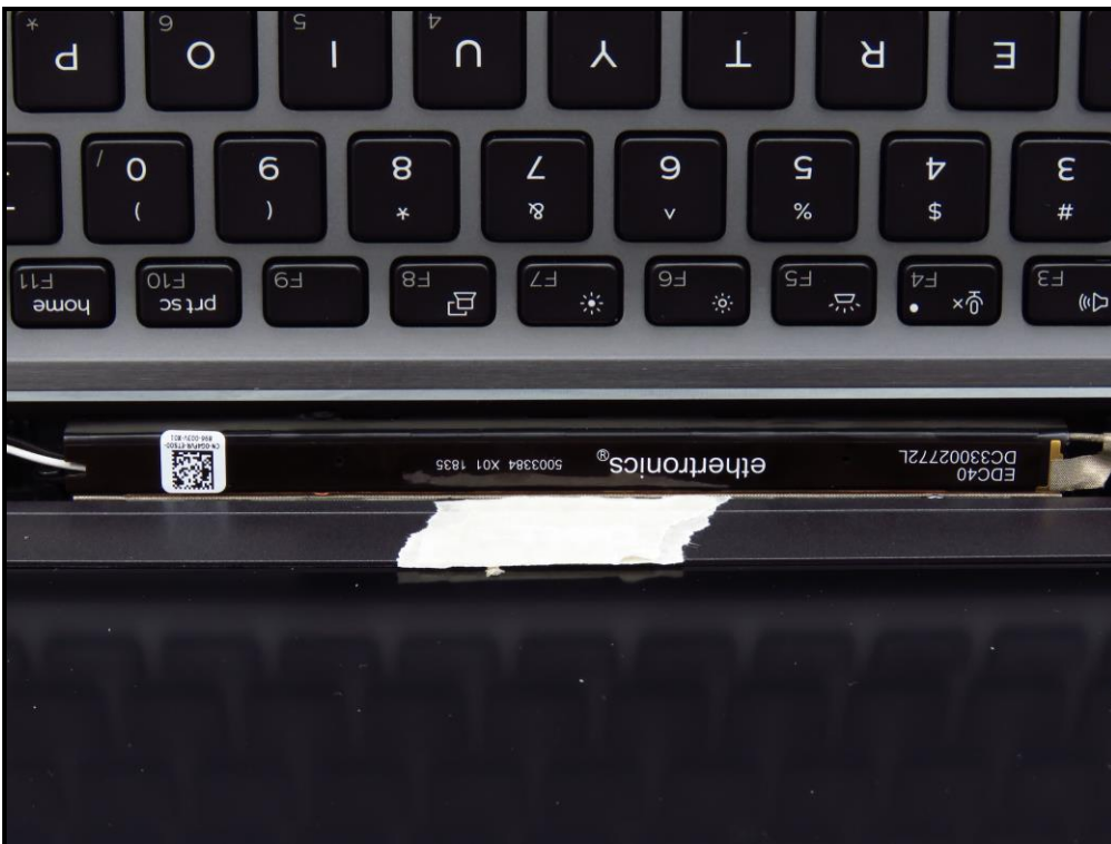
*ET antenna (material: AL)
