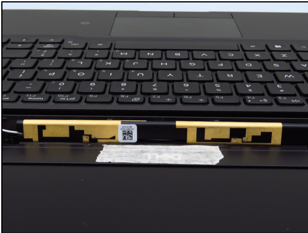
*WNC antenna (material: CF)
