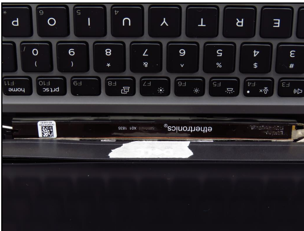
*ET antenna (material: AL)
