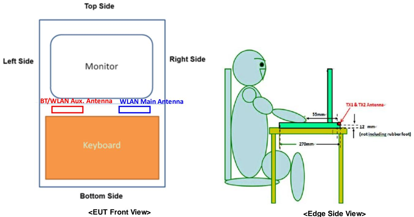
The separation distance for antenna to edge:
