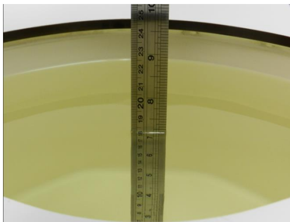
Fig 10.1 Photo of Liquid Height for Body SAR
