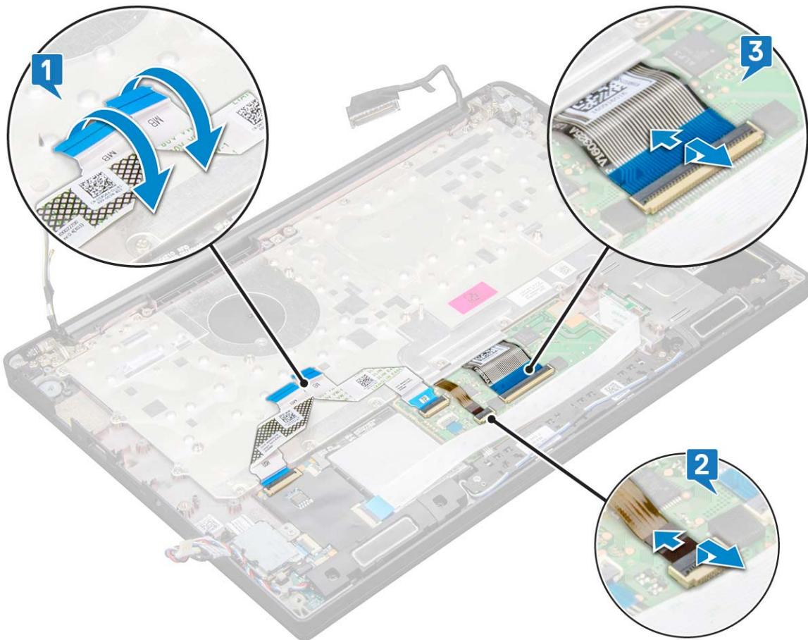
4 To remove the keyboard assembly:
