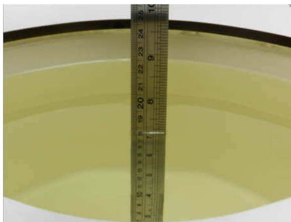
Fig 10.1 Photo of Liquid Height for Body SAR
