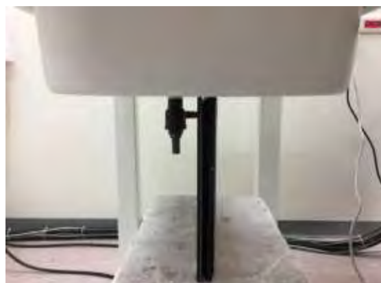
Fig.3 EUT Top side to flat phantom (tablet mode)
