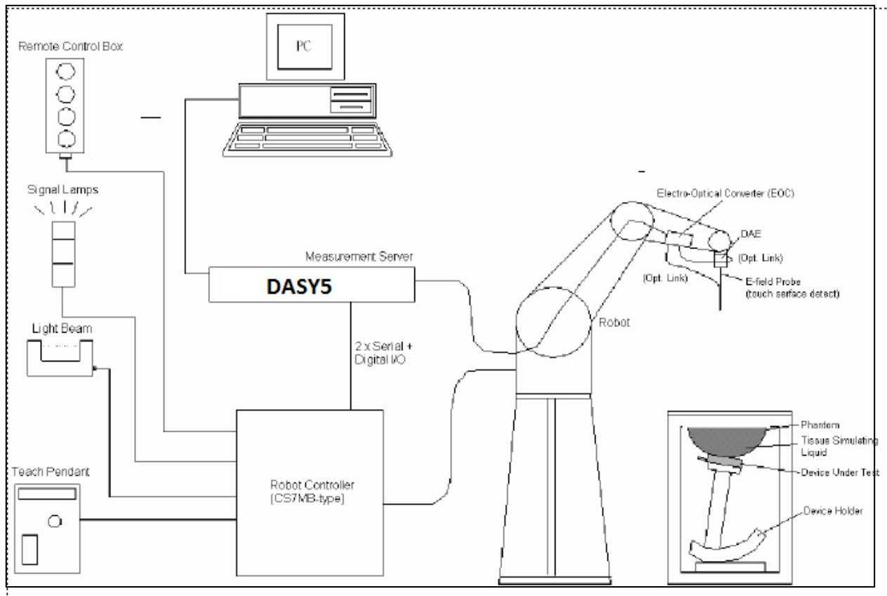
The DASY5 system for performing compliance tests consists of the following items:
