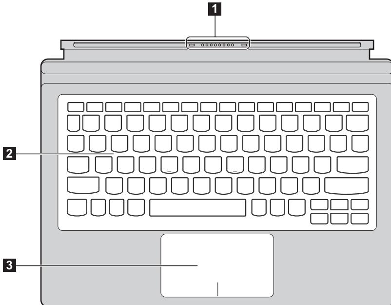
**1 Pogo pin with guide pin** Connect the tablet to the keyboard Folio and secure it in the installation position.
