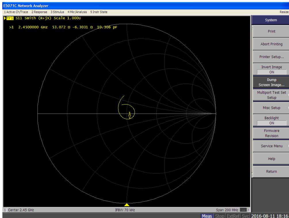
2450MHz Body calibrated return loss: -26.642 dB; Measured return loss: -26.245dB (within 20%)
