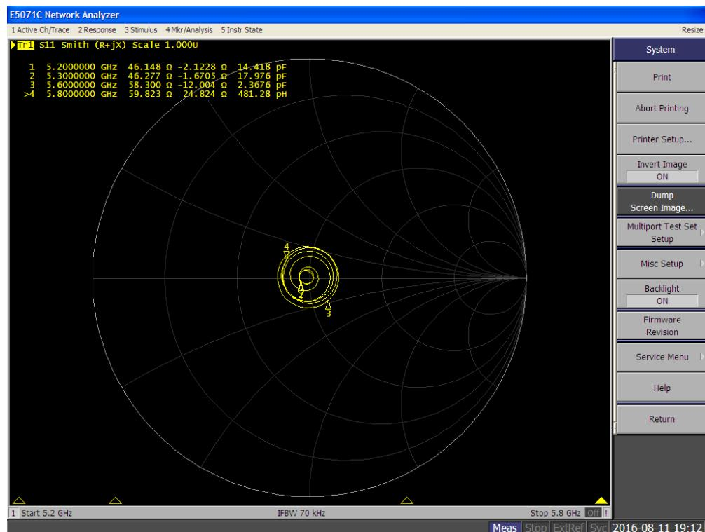
5200MHz Body calibrated return loss: -24.413 dB; Measured return loss: -20.805dB (within 20%)
