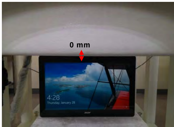
Fig.3 EUT Top side to flat phantom
