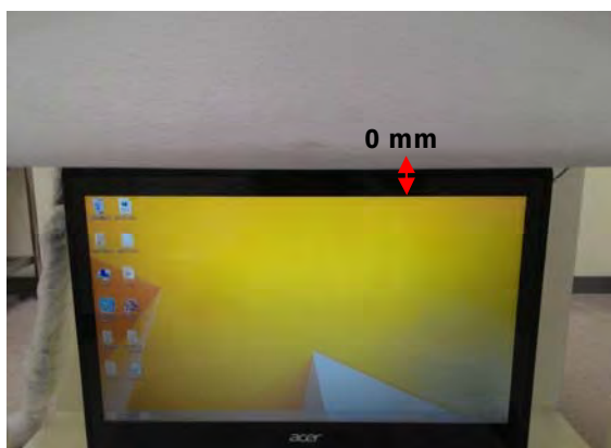
Fig.4 EUT Top side to flat phantom
