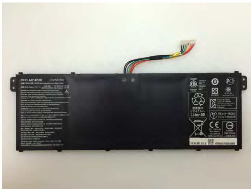
Fig.7 2 nd Battery (Model No.:AC14B3K, Supplier:Sanyo)
