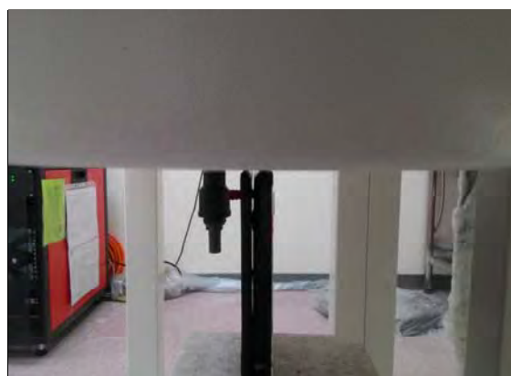
Fig.4 EUT Top side to flat phantom
