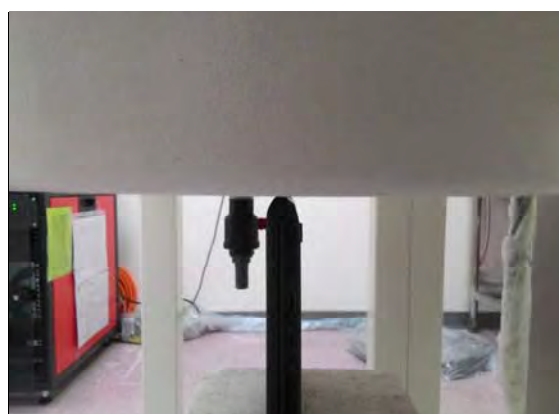
Fig.5 EUT Top side to flat phantom
