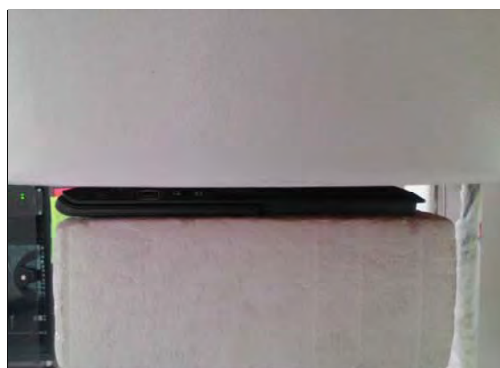
Fig.4 EUT Back side (Tablet) to flat phantom
