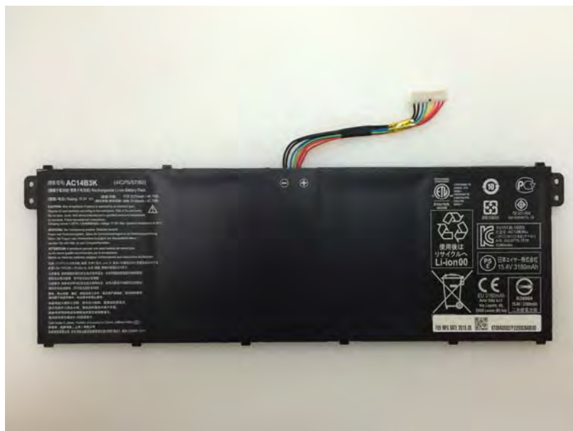
Fig.8 2 nd Battery (Model No.:AC14B3K, Supplier:Sanyo)
