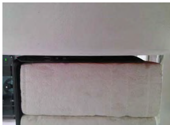
Fig.3 EUT bottom of keyboard touch flat phantom
