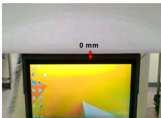
Fig.5 EUT Top side to flat phantom
