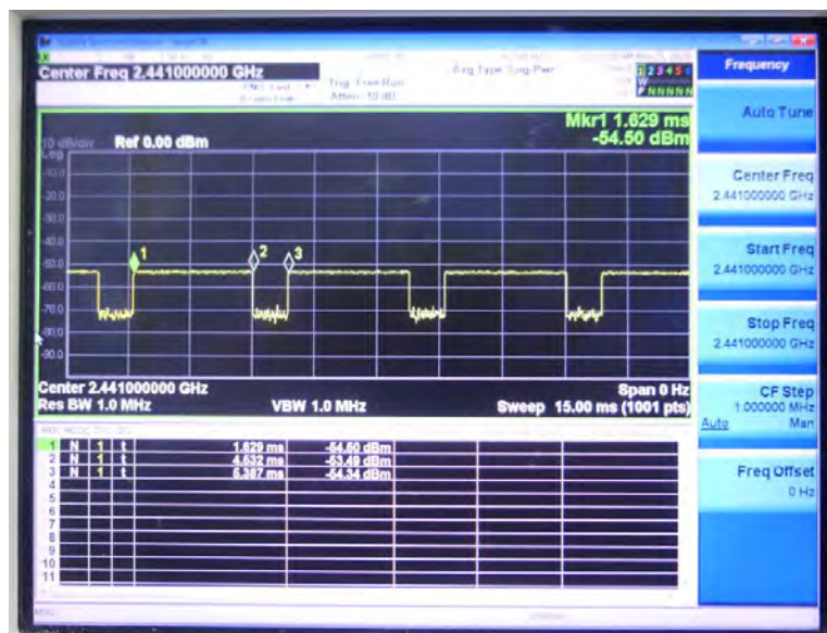
Time-domain plot for Bluetooth transmission signal
