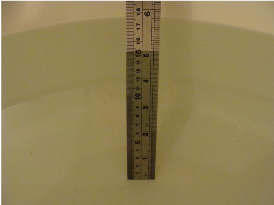
Depth of the liquid in the phantom-Zoom In (2.4GHz)
