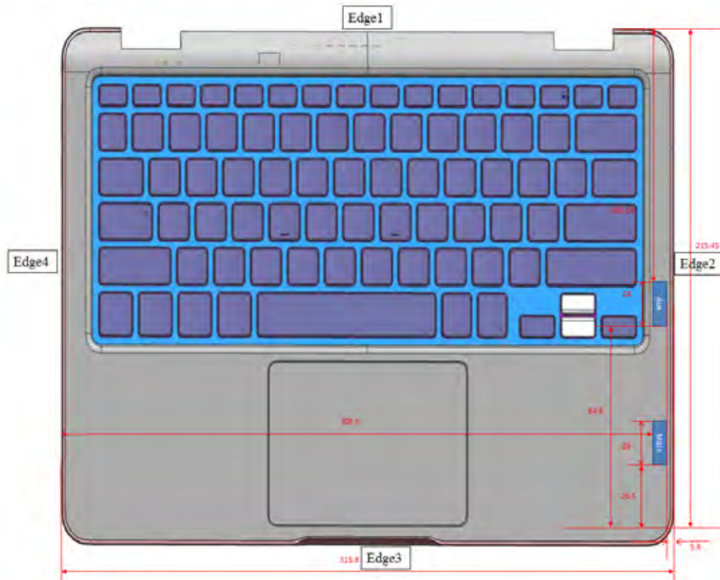
<The Distance information of Antenna to Edges of Tablet PC>
