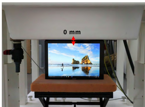
Fig.3 EUT Top side to flat phantom
