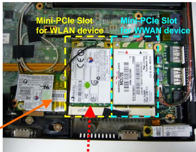
The certification label is stuck on the top side of the applying transmitter device, and the FCC ID is visible when the palm rest assembly is removed.
