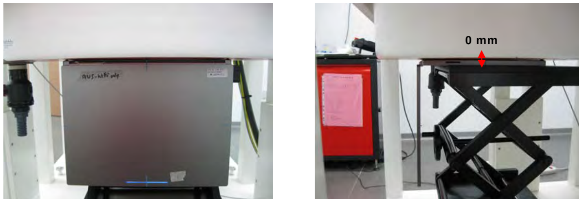
Fig.3 EUT Laptop mode to flat phantom
