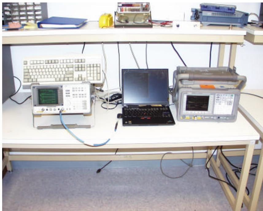
**TRANSMITTER RADIATED RF MEASUREMENT SETUP**
