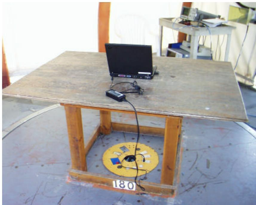
**DIGITAL DEVICE RADIATED EMISSIONS MEASUREMENT SETUP**
