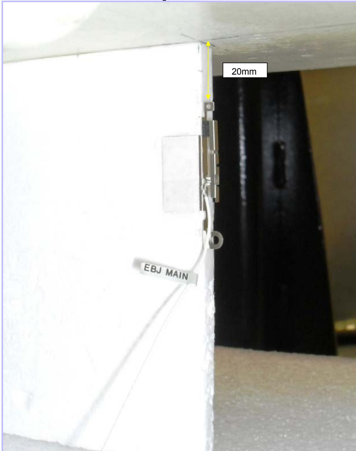
PHT/80583JD01/006: General Setup EUT in Horizontal-Up Facing Phantom
