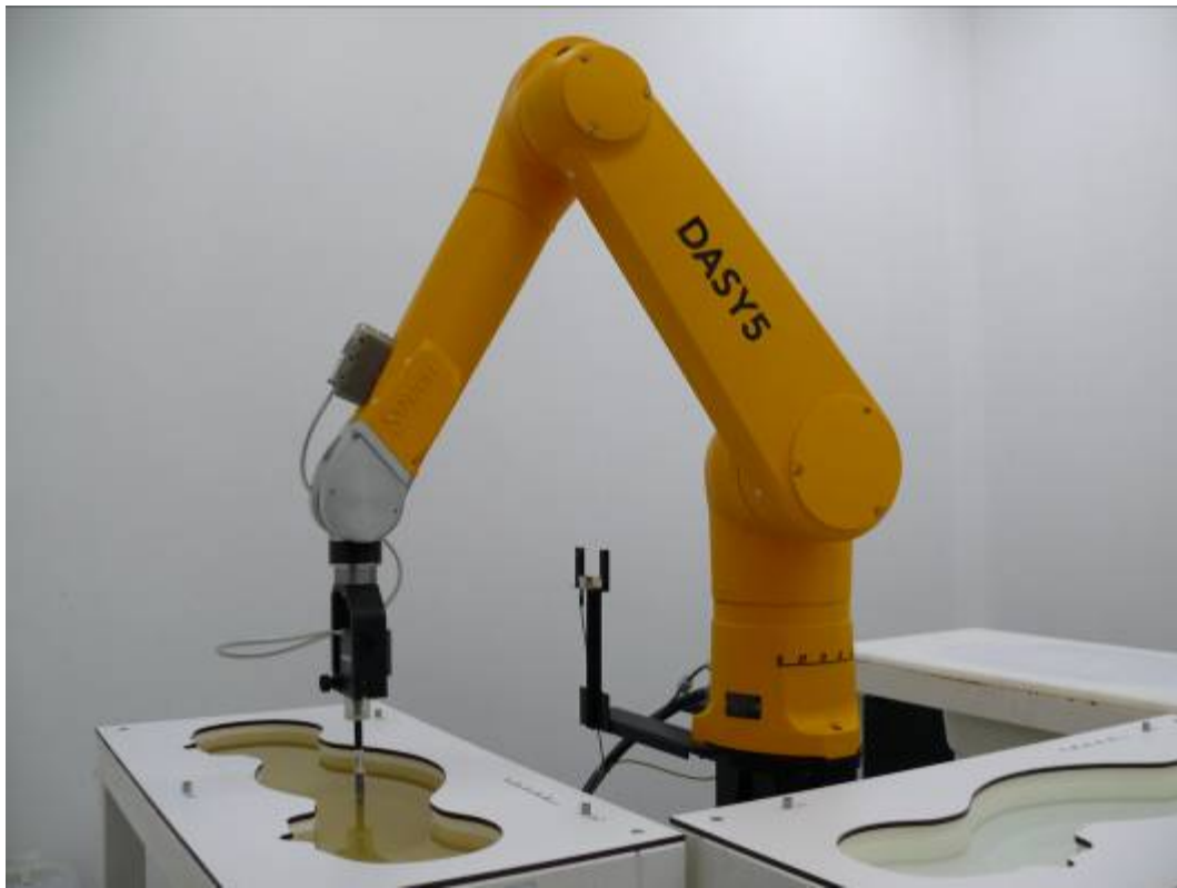
Picture 1: Specific Absorption Rate Test Layout
