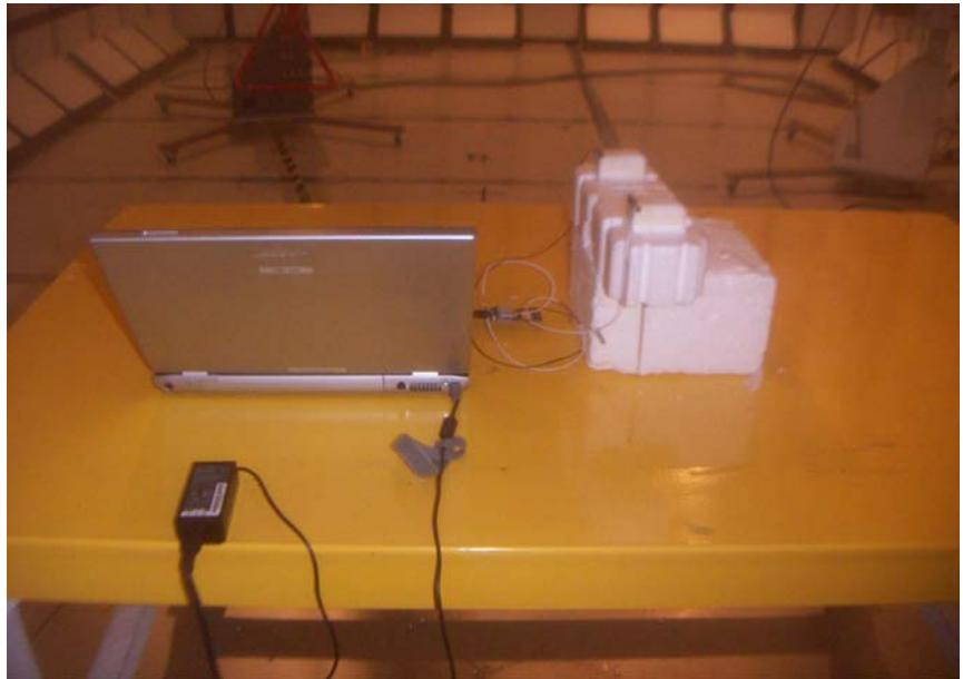
POWERLINE CONDUCTED EMISSIONS MEASUREMENT SETUP
