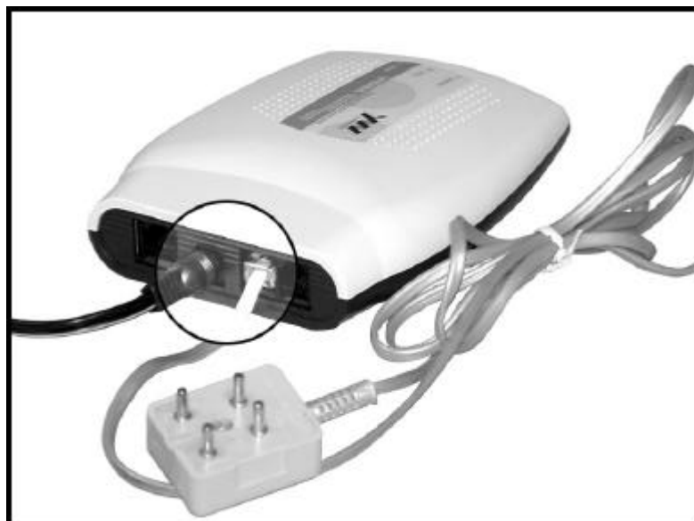
<Figure 10> Connecting phone line to modem
