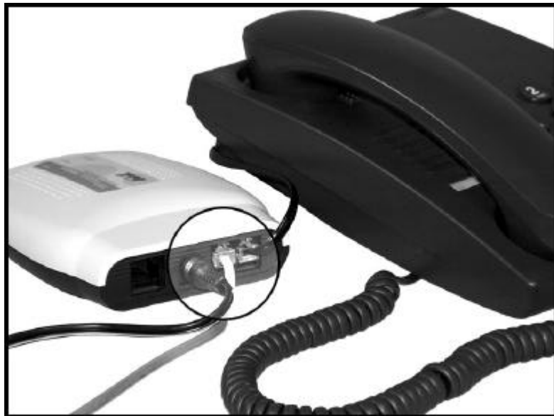
<Figure 11> Connecting phone line to modem
