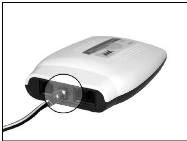
<Figure 12> Connecting Power Code
