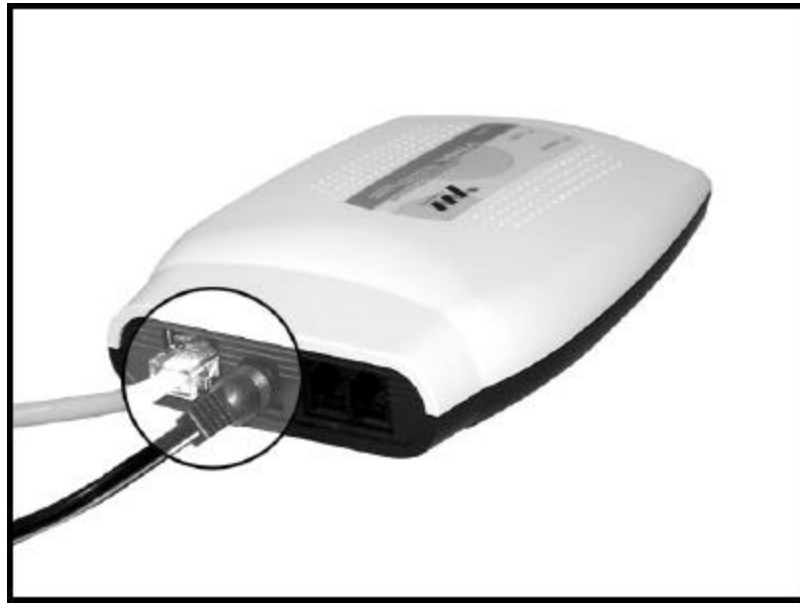
<Figure 9> Connecting Ethernet Cable to Modem
