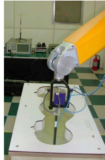
Figure 4. Photograph of the probe and the Phantom
