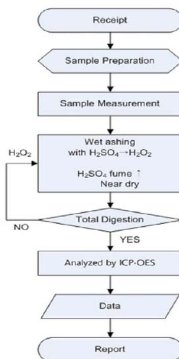
\*\* Remarks : The samples were dissolved totally by pre-conditioning method according to above flow chart.
