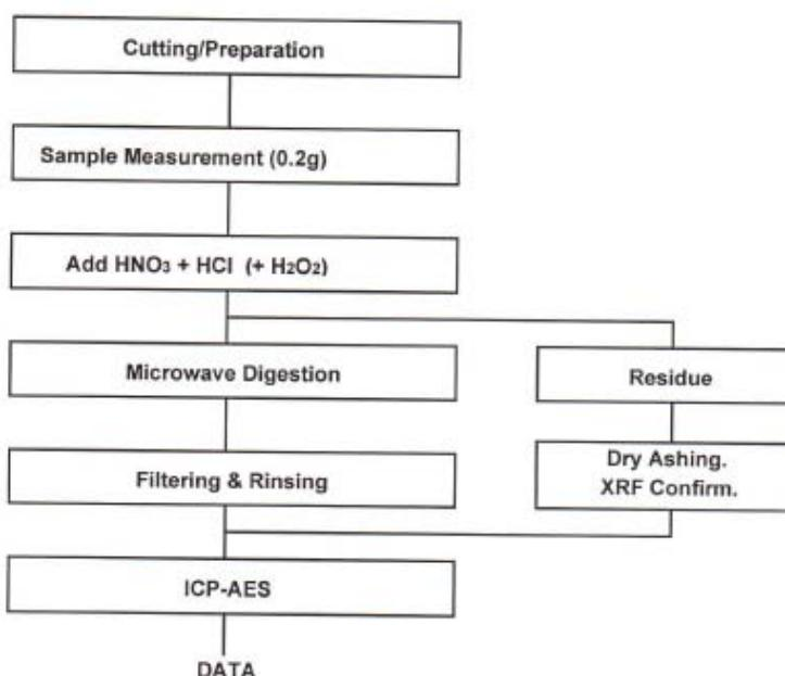
The samples were dissolved totally by pre-conditioning method according to above flow chart.
