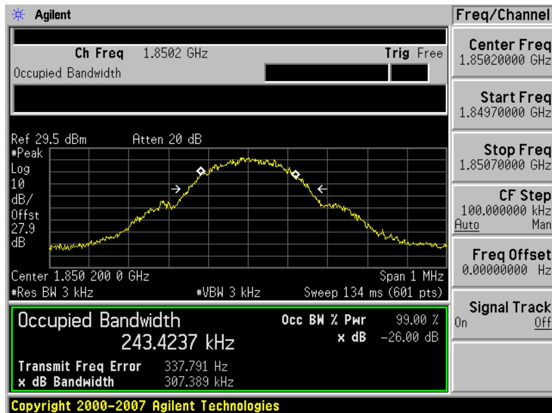
■ GSM1900 MODE (661 CH.) Occupied Bandwidth
