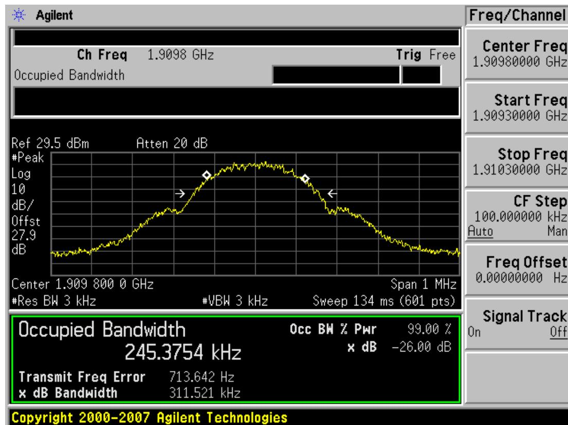
■ GSM1900 EDGE (661 CH.) Occupied Bandwidth
