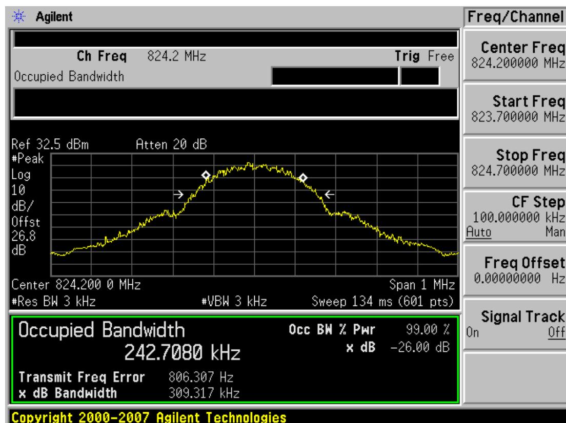
■ GSM850 MODE (190 CH.) Occupied Bandwidth
