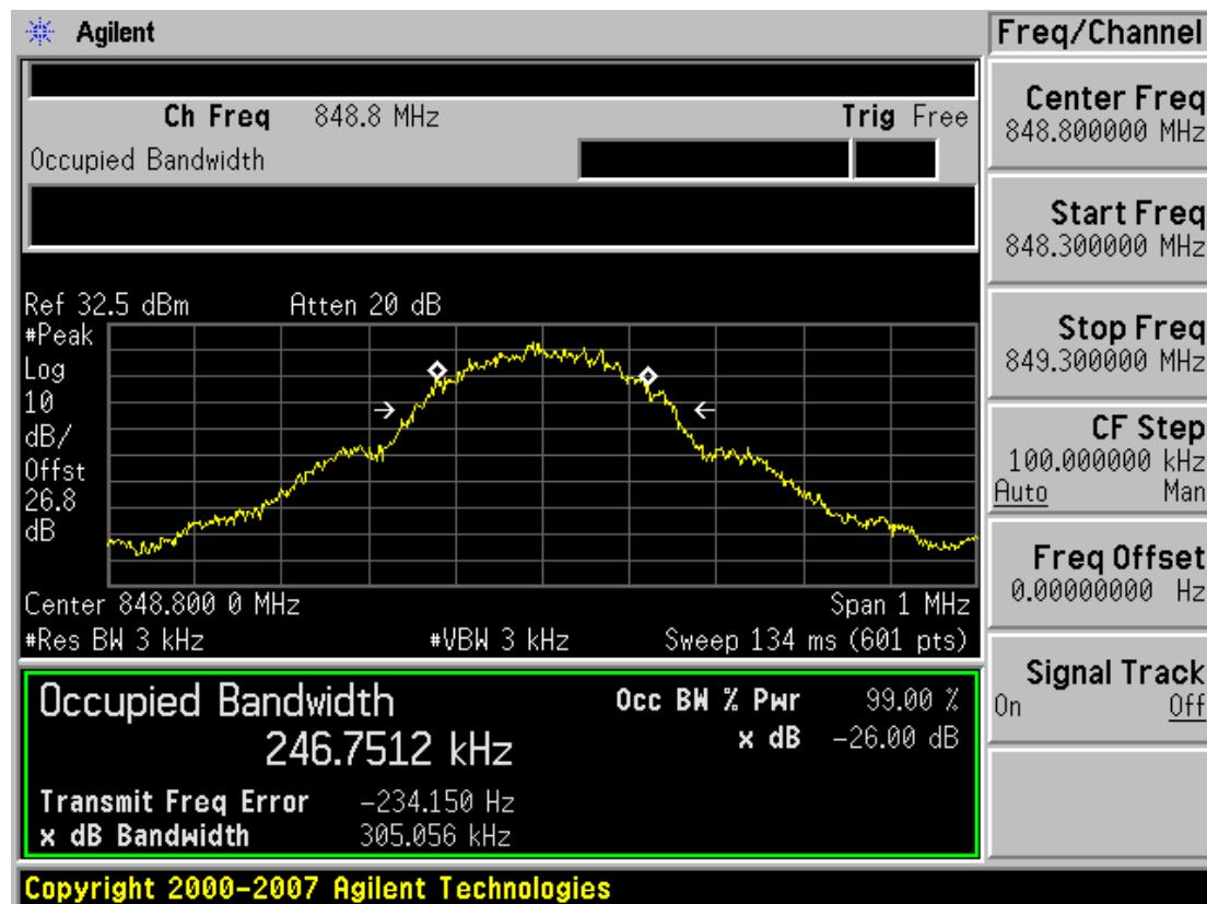
■ GSM850 EDGE (251 CH.) Occupied Bandwidth
