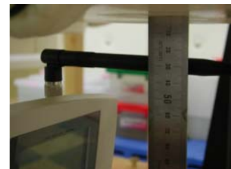
Fig. 21. Body SAR Test Setup with Holster
