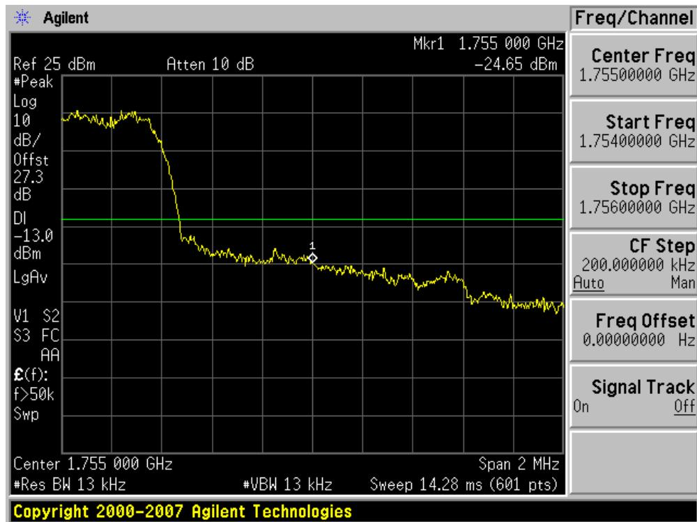
■ AWS CDMA MODE (25 CH.) 4MHz Span
