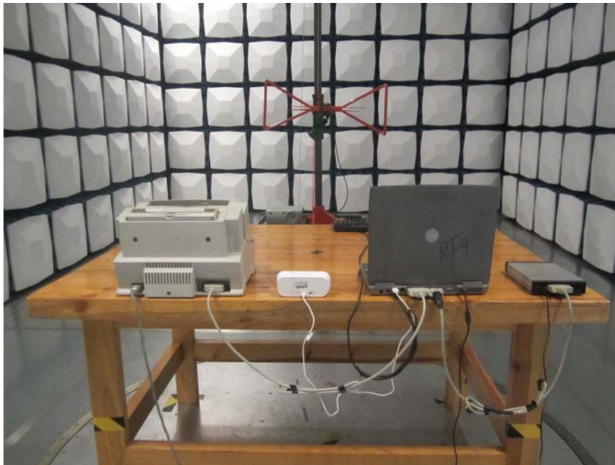
Radiated Emission - Below 1GHz Rear View
