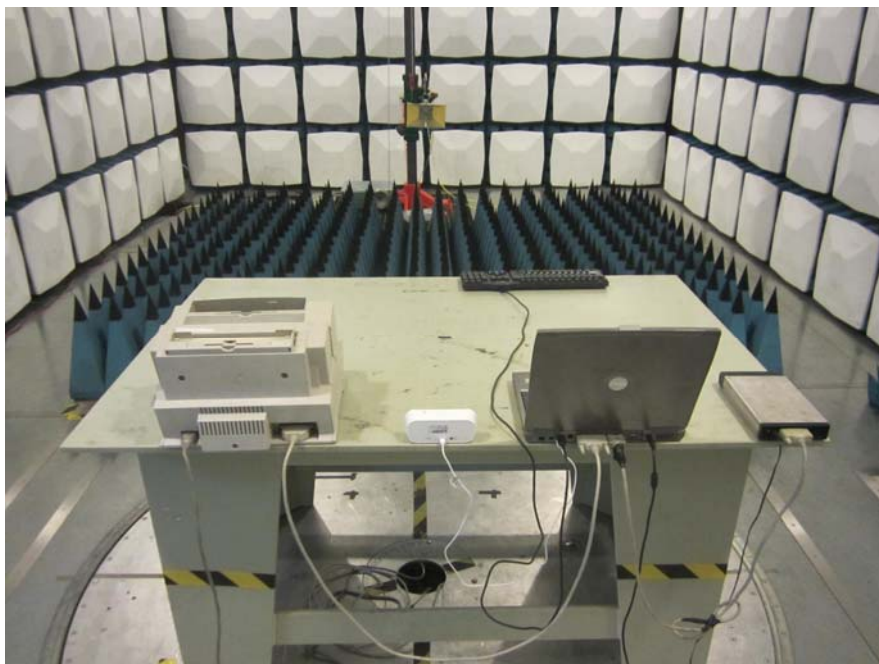
Radiated Emission - Above 1GHz Rear View
