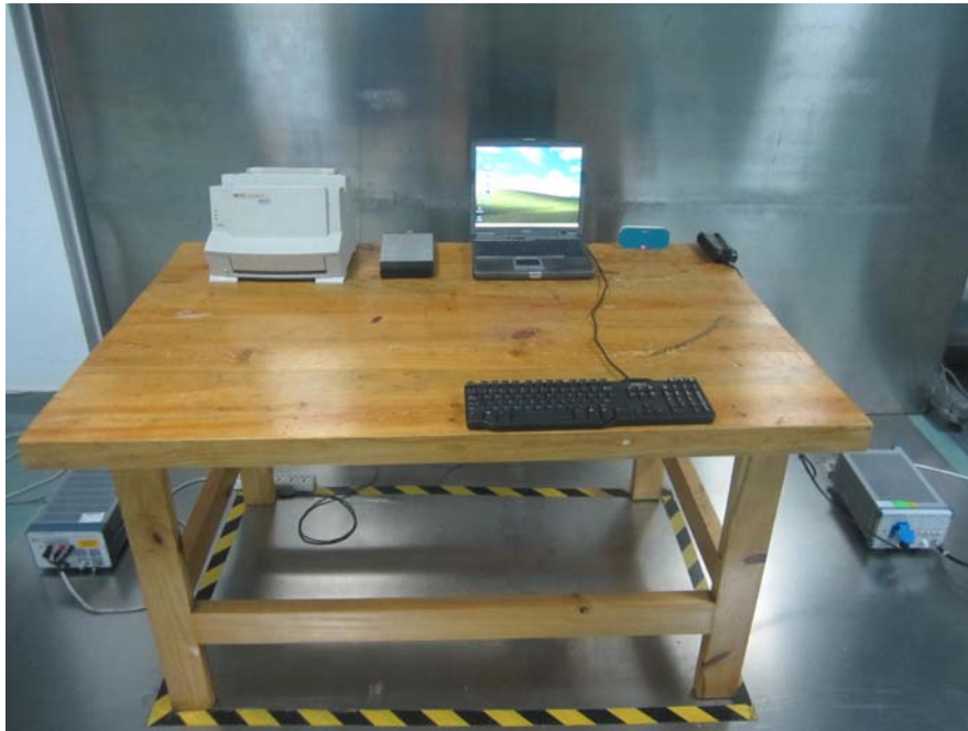
Conducted Emissions - Front View
