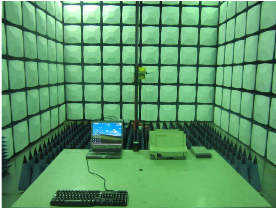
Radiated Emission - Above 1GHz Front View
