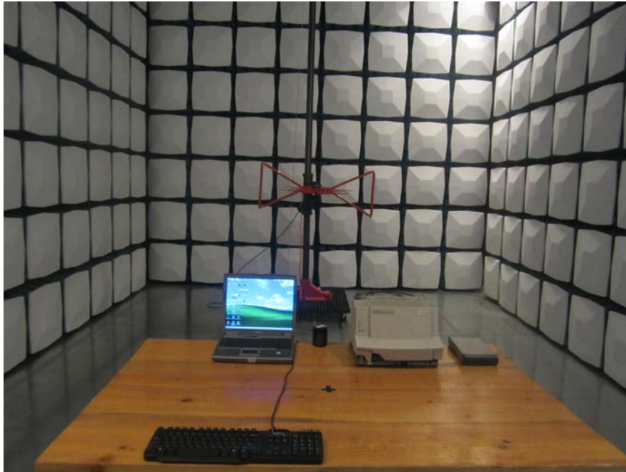
Radiated Emission - Below 1GHz Rear View
