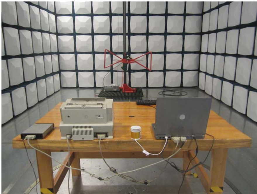
Radiated Emission - Below 1GHz Rear View
