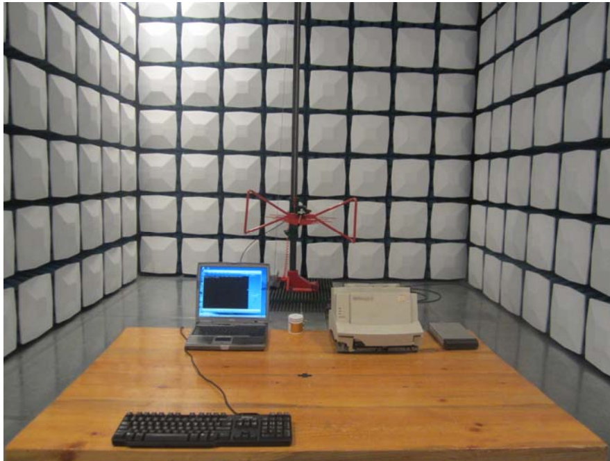
Radiated Emission - Below 1GHz Front View
