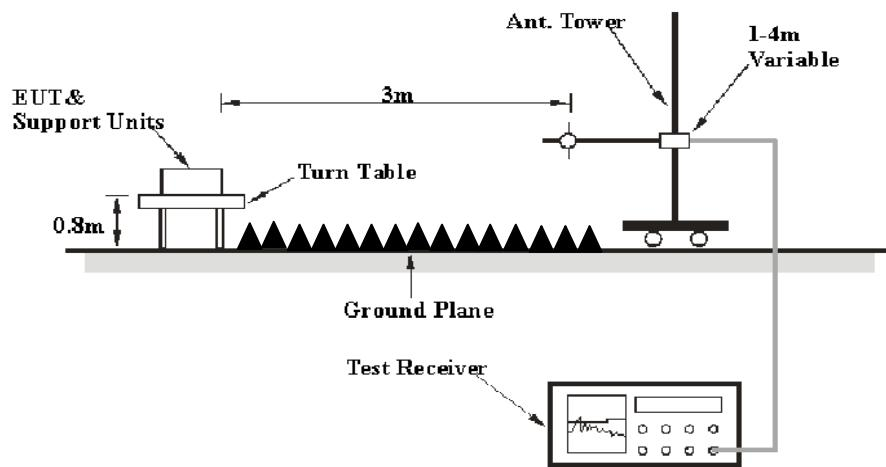
The radiated emission and out of band emission tests were performed in the 3 meters chamber test site, using the setup accordance with the ANSI C63.4-2003. The specification used was the FCC 15.209/15.205 and FCC 15.249 limits.
