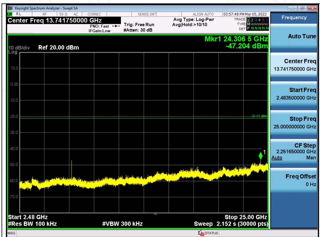
Test_Graph_GFSK_ANT1_2402_Higher Band Emissions
