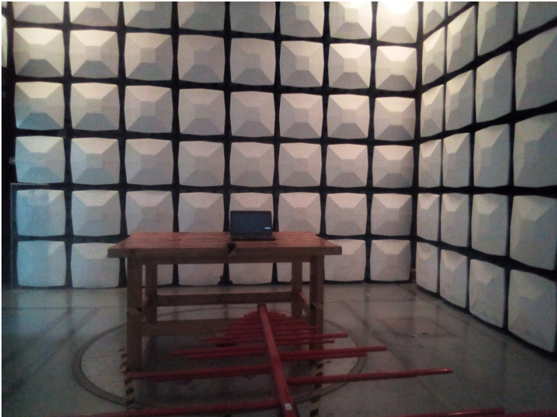
RE Below 1G front View
