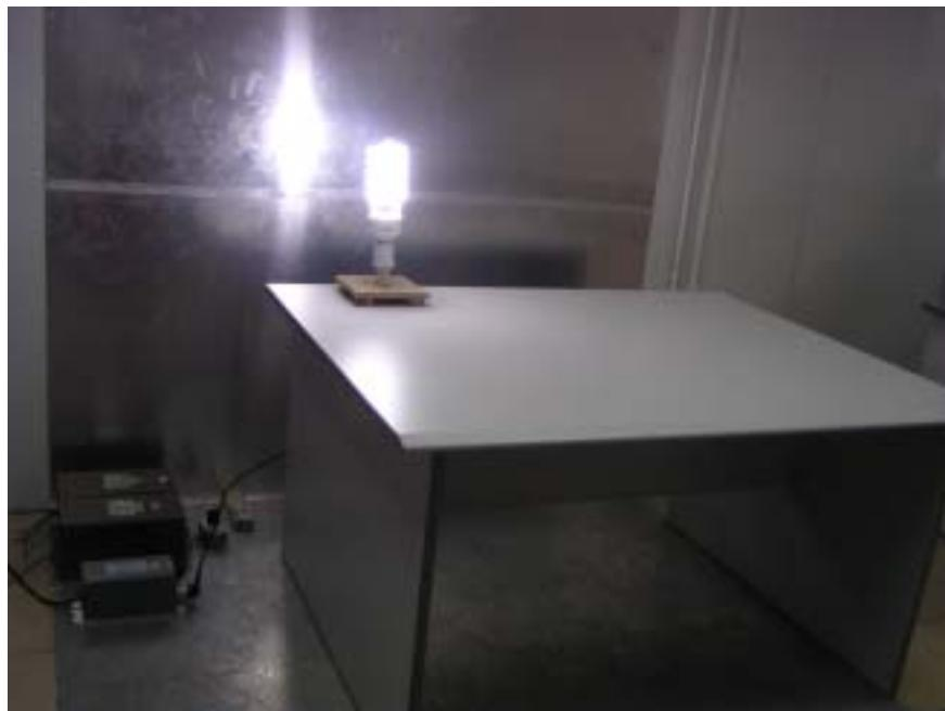
Conducted Emission of SUS-85W – Side View
