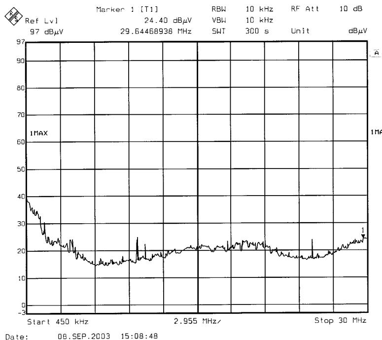
The plot of conducted emission tested with Commercial Electric power cord extension, M/N: SUN-15W was presented hereinafter as reference.
