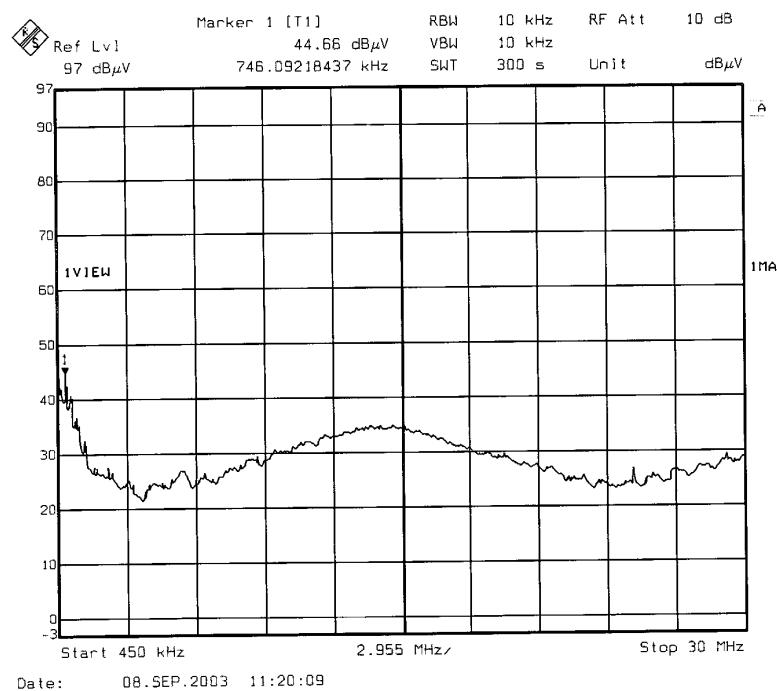
The plot of conducted emission tested with Commercial Electric power cord extension, M/N: SUS-65W was presented hereinafter as reference.
