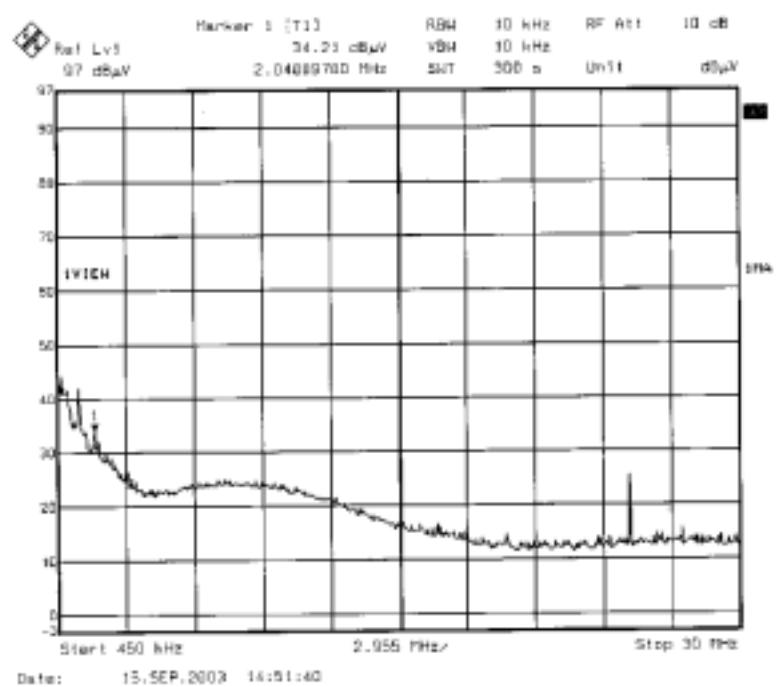
The plot of conducted emission tested with Commercial Electric power cord extension, M/N: SUS-85W was presented hereinafter as reference.
