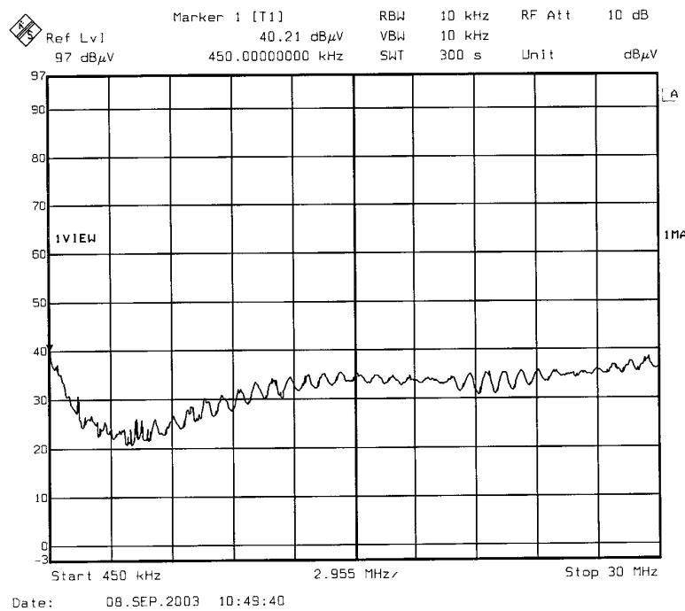
The plot of conducted emission tested with Commercial Electric power cord extension, M/N: SUS-55W was presented hereinafter as reference.
