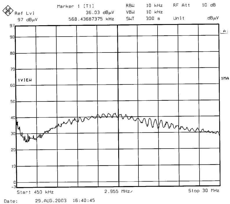
The plot of conducted emission tested with Commercial Electric power cord extension, M/N: TUW-28W was presented hereinafter as reference.
