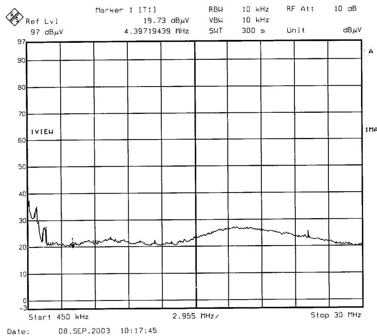
The plot of conducted emission tested with Commercial Electric power cord extension, M/N: EUM-11W was presented hereinafter as reference.
