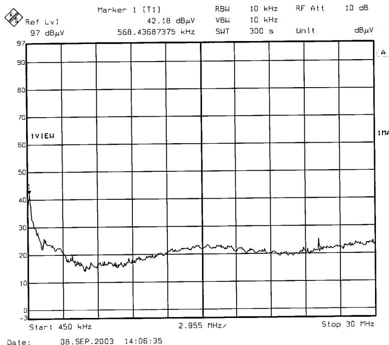
The plot of conducted emission tested with Commercial Electric power cord extension, M/N: SUS-105W was presented hereinafter as reference.
