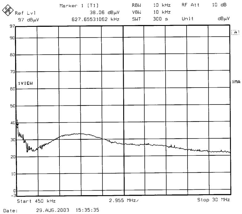
The plot of conducted emission tested with Commercial Electric power cord extension, M/N: SUN-20W was presented hereinafter as reference.
