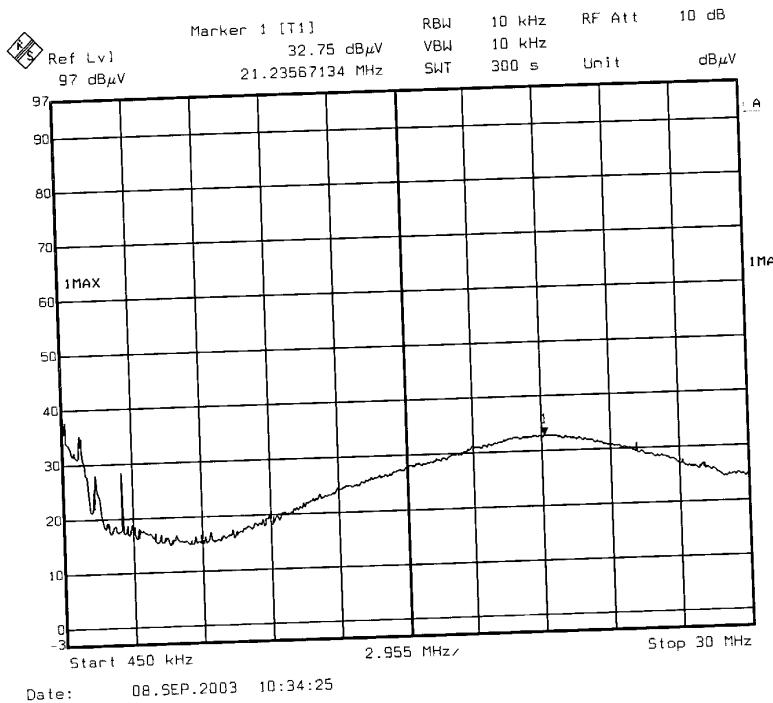
The plot of conducted emission tested with Commercial Electric power cord extension, M/N: SUN-24W was presented hereinafter as reference.
