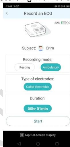
1) Recording time is available from one minute to 24 hours (below image). A result is shown for every minute of recording (no result available for recording less than one minute).
