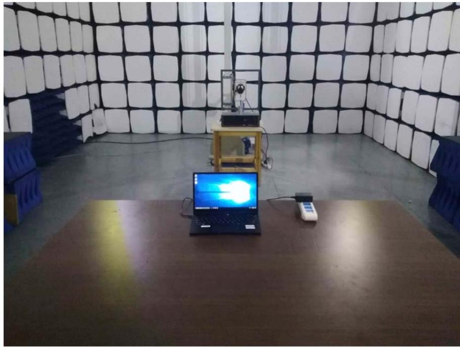
**Radiation Emission Test Setup (30MHz to 1GHz)**
